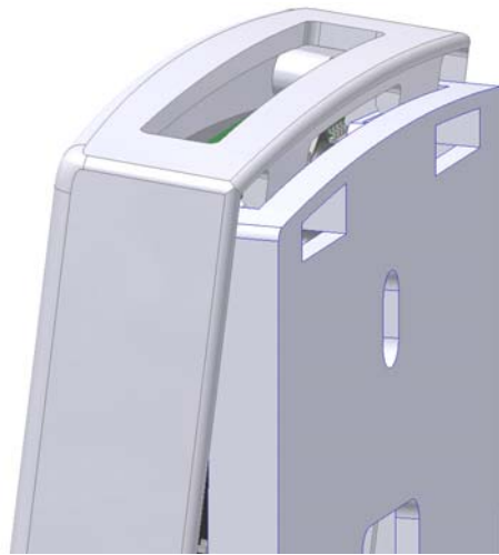
Figure 7.3.3, Top Cover Mounting Tabs and Top Base Mounting Slots
