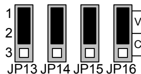
Figure 2.18 Jumper shunt positions for interfacing with a voltage output.
